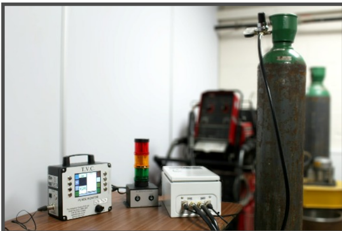
GPM unit set up with Flow Control Regulator Box
