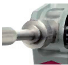
Eccentric plate triples the use of the diamond wheel
