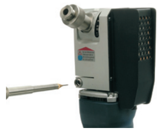
Precise adjustment of the stick-out
